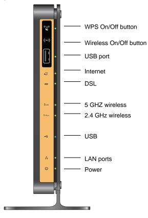
Figure 4. Front panel LEDs
